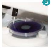
As the agar plate spins, the syringe automatically dispenses accurate volumes of sample.
