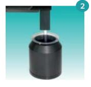
The syringe takes the liquid sample from an irradiated sample beaker.
