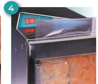
4 Pick up the bag with the homogenized sample ready to be analyzed.
