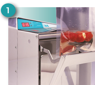
1 Introduce the sample into the sterile bag.
