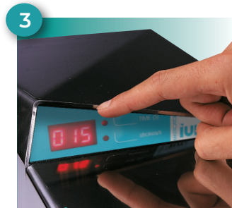
3 Set the parameters and start the process closing the door.
